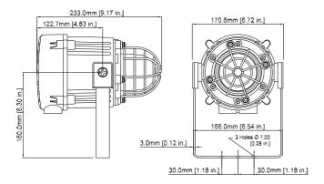
Fig. 1 Fixing Location for Beacon
