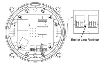
Fig. 8b End of Line Resistor Placement
