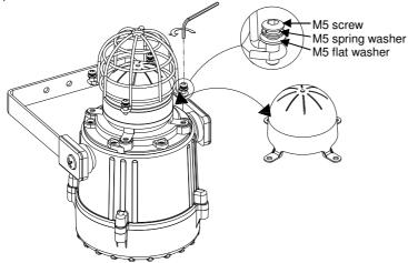
Fig. 9 Replacement of beacon lens cover
