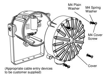
Fig. 2 Accessing the Enclosure.
